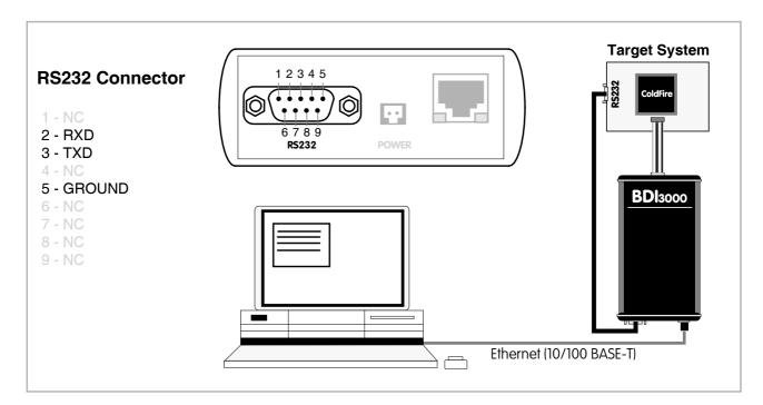
The configuration parameter "SIO" is used to enable this serial I/O routing. The used framing parameters are 8 data, 1 stop and not parity.
