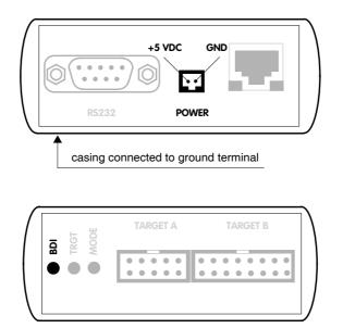
The green LED «BDI» marked light up when 5V power is connected to the BDI3000
